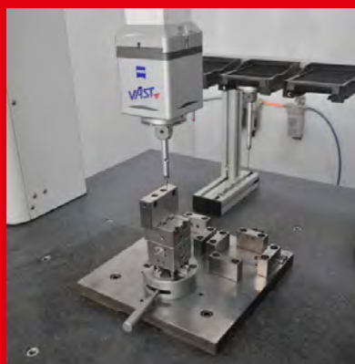
ZEISS三坐标测量仪检测 3A-200002旋转摆动式虎钳 ZEISS coordinate measuring machine detects Rotatable Pendulum Vise 3A-200002
